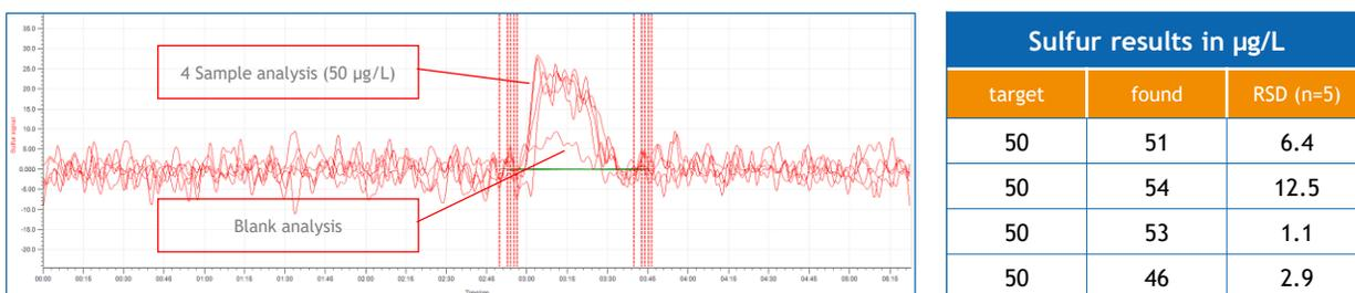
Figure 7A: Overlay of multiple analysis of a 50 µg/L Sulfur standard analyzed as sample and a blank
