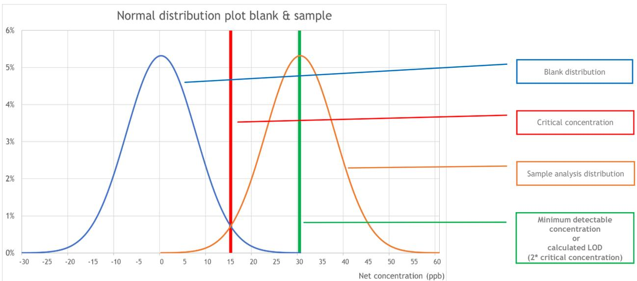
Figure 4: Normal distribution plot minimum detectable value (or LOD)
