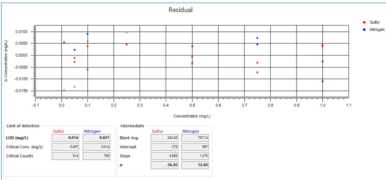
Figure 6: Residual plot for 0-1 mg/L S & N calibration
