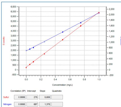
Figure 5C: Calibration curve 0-1 mg/L for both Sulfur & Nitrogen
