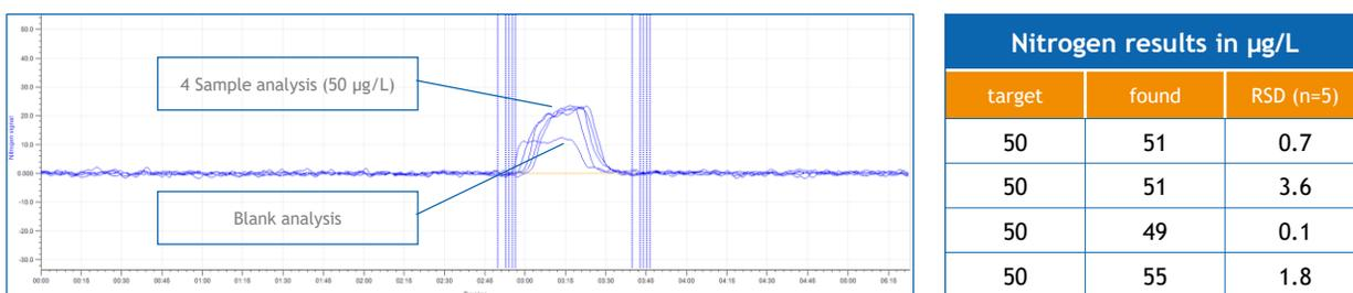
Figure 7B: Overlay of multiple analysis of a 50 µg/L Nitrogen standard analyzed as sample and a blank
