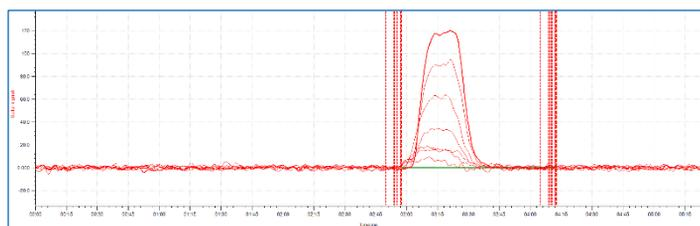
Figure 5A: Overlay of Sulfur 0-1 mg/L calibration analysis
