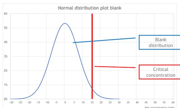
Figure 2: Normal distribution plot of multiple blank analysis
